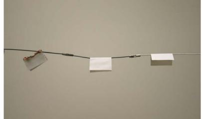
Figure 2: With the Variac output at ~90 V, the paper on the Nichrome wire (far left) burns and falls off. The paper on the steel wire (middle) and the copper wire (far right) are unchanged. (Note that the copper wire has a tin coating.)
