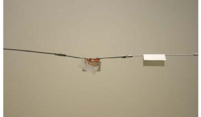
Figure 3: With the Variac output at  $\sim$ 115 V, the paper on the steel wire burns and falls off. The paper on the copper wire is unchanged.
